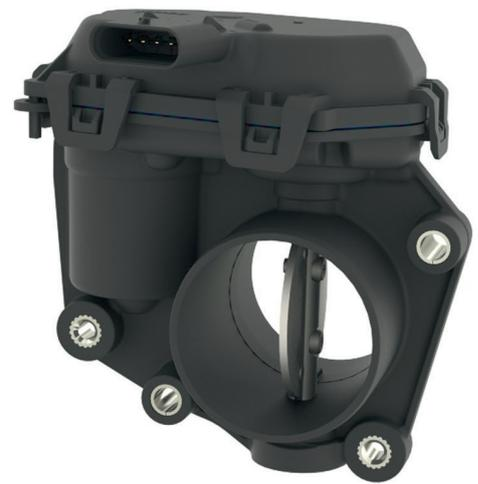
**Fig. 5.** Picture of the finished component: the housing of an electromechanical actuator made of PBT. It is lighter by 35 % compared to aluminum in this design. © Valeo/Hofmann
