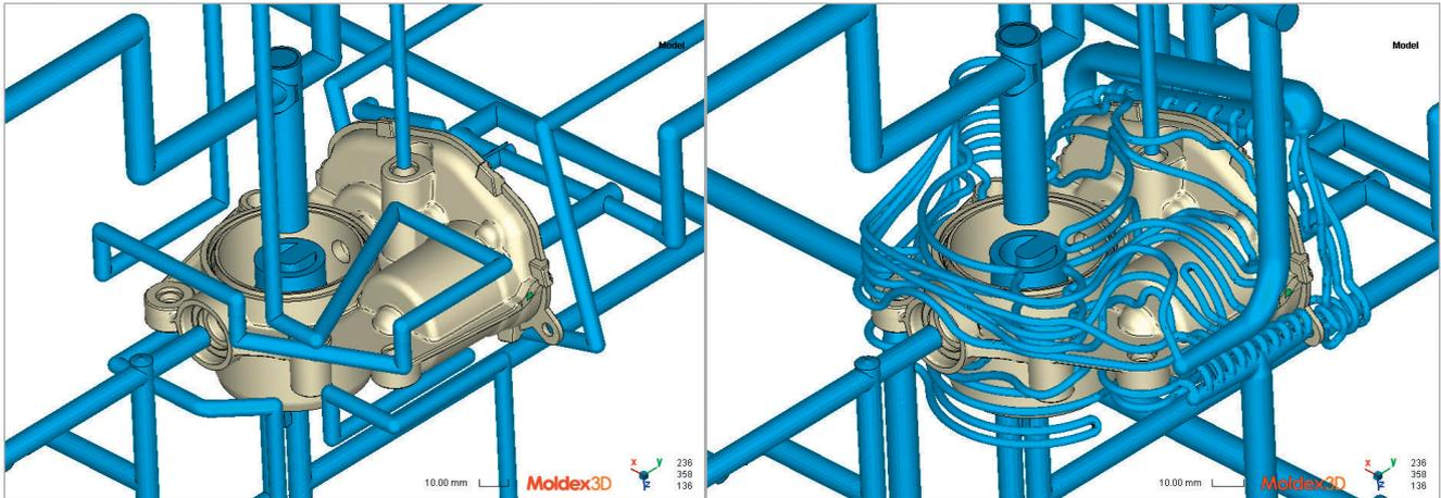
**Fig. 1.** Left: conventional cooling (blue) and component (beige). Right: conformal cooling channels from additive manufacturing and component.
