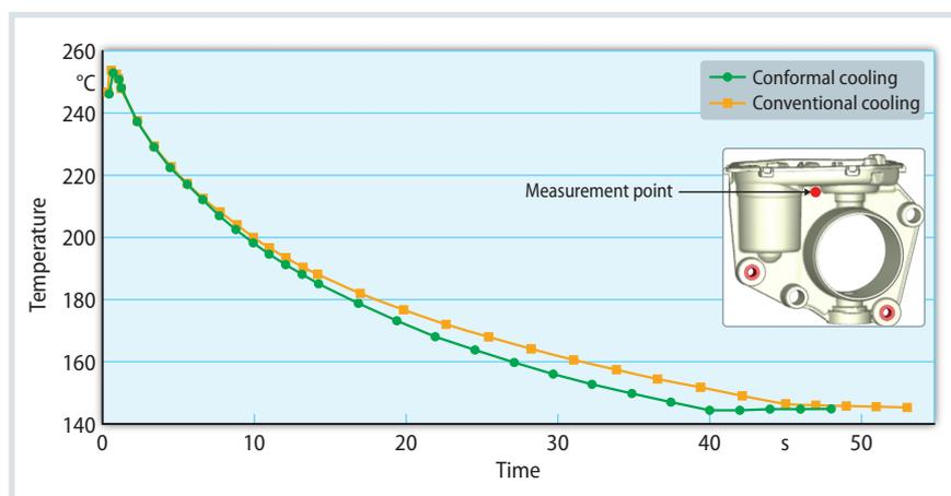
**Fig. 4.** Comparison of the surface temperature at the back of the hotspot for conformal and conventional cooling. Source: Valeo/Hofmann; graphic: @ Hanser
