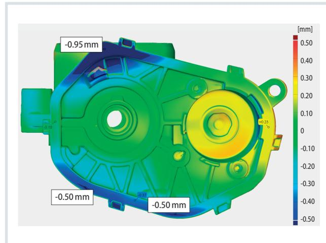
**Fig. 2.** Top view of the housing. The warpage of the component after simulation with conformal cooling at the interface to the cover is visualized.
