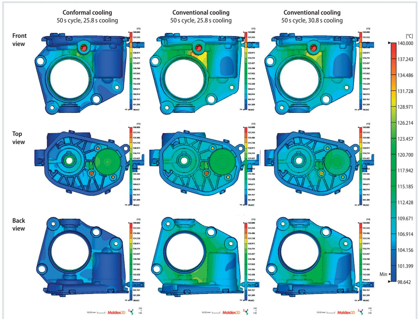
Fig. 3. Comparison of surface temperatures at the end of the cycle for different cooling methods. Source: Valeo/Hofmann; graphic: @ Hanser
